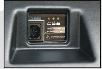
High frequency battery charger built-in with battery charge indicator and block of the forks with flat battery
