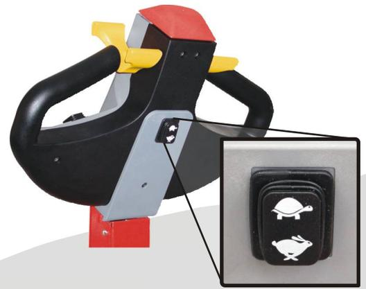
Speed Selector to operate with the tiller in the upright position
