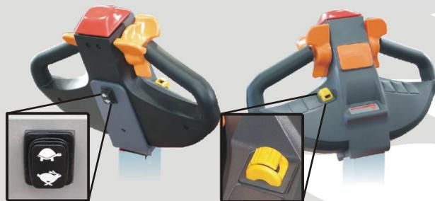
Roller to control the lifting + descending speed of the Forks
